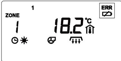
**Battery error:** Battery low or discharged. Replace the battery immediately. The battery is located inside the control unit cover. Type: 1.5V (AA). Use long-life batteries. Before changing the batteries please read the general security instructions – and in particular Section 4.4.4!
