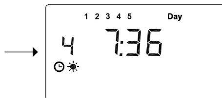
In this case a new switch point was programmed with a time of 7:35. This time parameter was used previously in switching point 3. Thus the time for point 4 changes automatically to 7:36.
