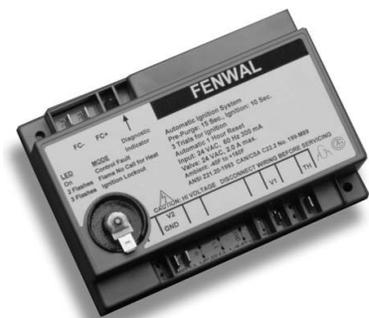
If the established flame signal is lost while the burner is operating, the control will respond within 0.8 seconds. The HV spark will be energized for a trial ignition period in an attempt to relight the burner.
