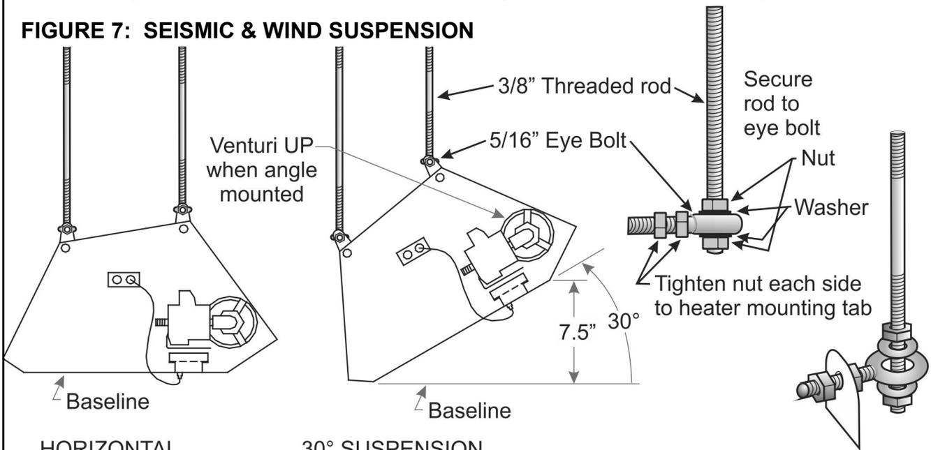
Measure to Base Point from any horizontal surface. At 30° mounting angle, the 'upper edge' is 7.5" higher than the Base Point
