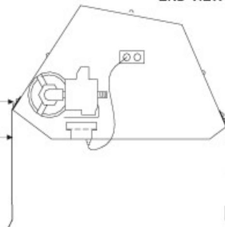
ATTACH REFLECTOR EXTENSION TO DRILLED SCREW HOLES
