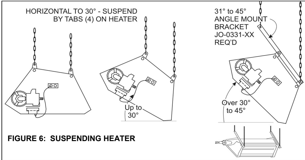
**FIGURE 6: SUSPENDING HEATER**
