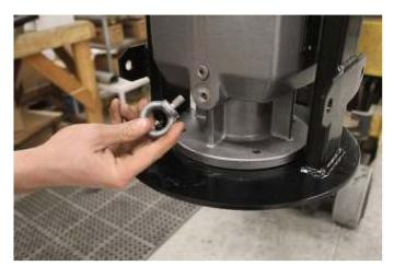
2. Place oil pan under drain plug, supporting oil pan properly.
