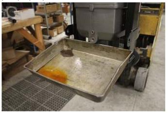
3. Remove drain plug using 6mm allen key.
