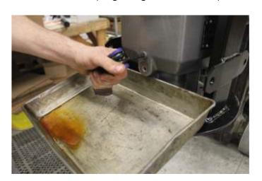
**4.** On right side of gearbox remove the fill plug in upper right corner using 6mm allen key.
